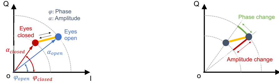
(a) The signal variation between the eye open and closed status. (b) The resultant phase and amplitude changes.
